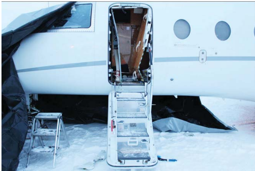
Post-accident view of the aircraft's main entrance door
